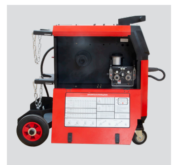
Wire support for coils up to 15 kg
