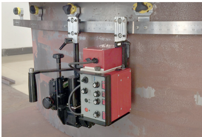
Tractor drive on Flexible steel-rail
