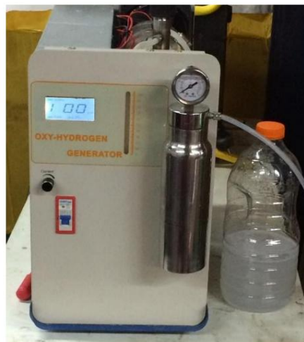
Figure 9 Setup OH generator
