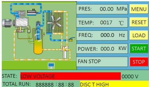
**NOTICE:** The compressor will not run if any alarm shows on the screen. Press the reset button before "START" button after the alarm has been corrected.
