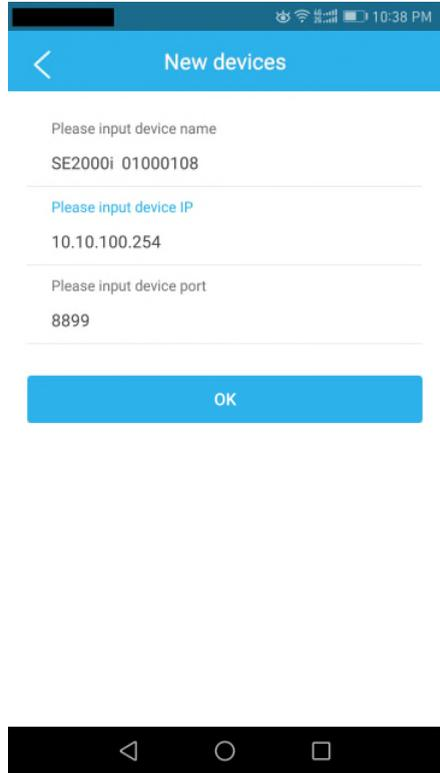
2.4 Before you click on "OK" in the "New devices" page, you will need to turn off the WLAN first but keep the page on. Then open the mobile network, to make sure mobile phone can connect to the mobile network, and then click "OK" in the "New devices" screen. You can see "add success" tip, the generator has been added into the APP.
