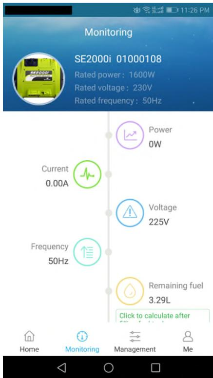
4.2 When you connect to the generator and do the monitoring, the generator picture and the Gen-mate serial number will be shown at the bottom of "Home" page.
