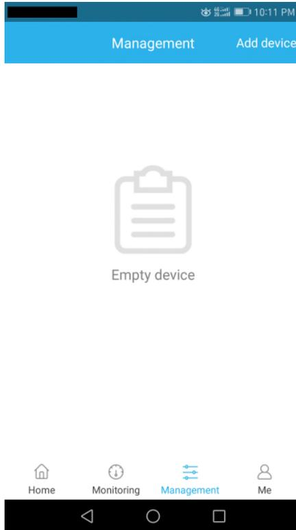
2.3 Click on "Add device", choose the WIFI signal that matched with your generator model in "Devices detected" page, click on the "Quick Add" on the right side of the signal.
